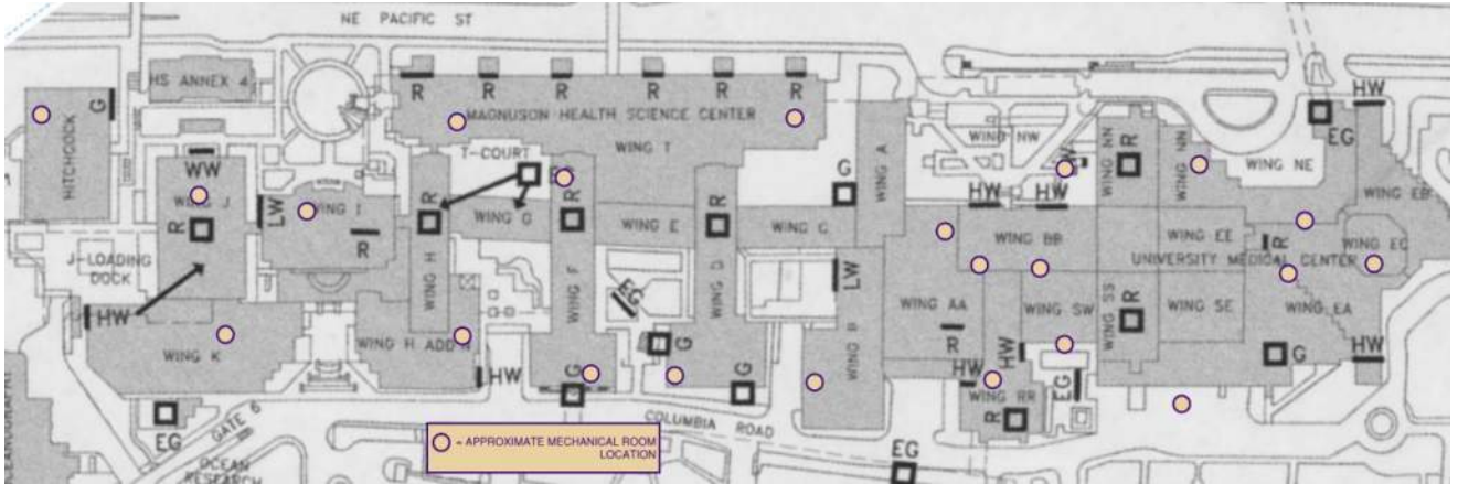
Figure 4.3.2-7: Vicinity Map of MHSC and UWMC with mechanical room locations identified in plan view
