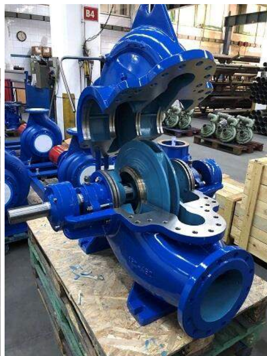
Figure 3-17. Photos of a horizontal split case pump assembled (left) and disassembled (right).
