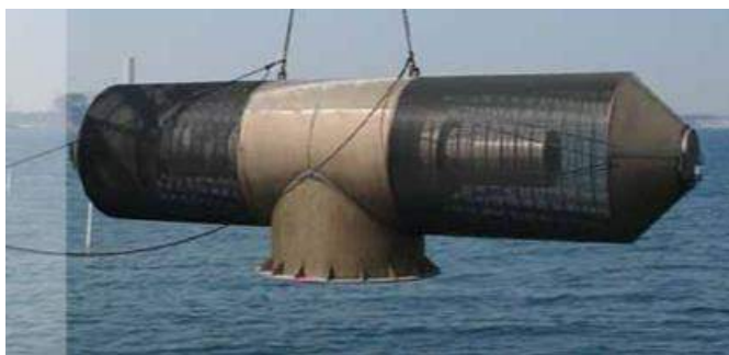
Figure 3-23. Photo of a T-screen, courtesy of Johnson Screens.
