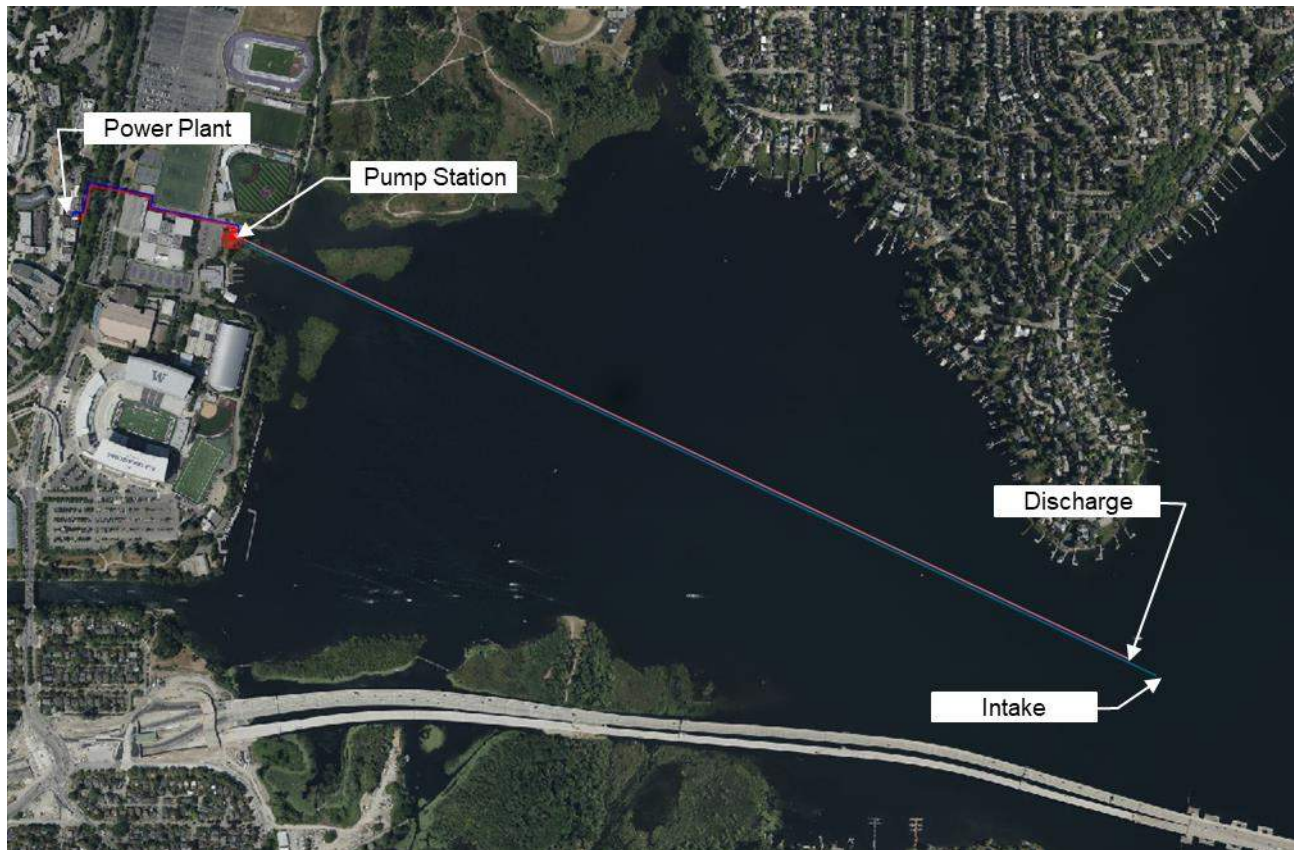
Figure 3-10. Plan view of the Return-to-Lake system configuration 1.
