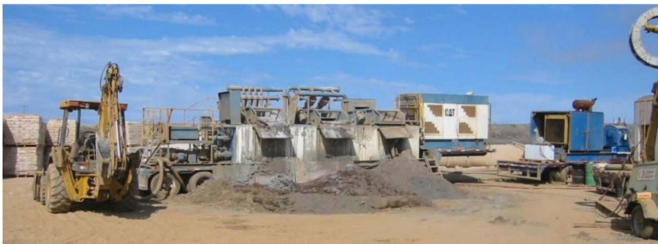
Figure 3-34. Typical drill fluid cleaner and pump system
