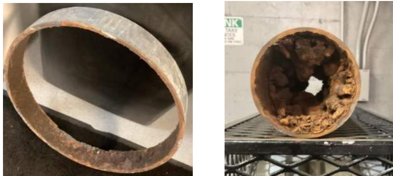
Figure 3.4.3-1: Sample of Power Plant tower water piping (left) and domestic water piping (right).
