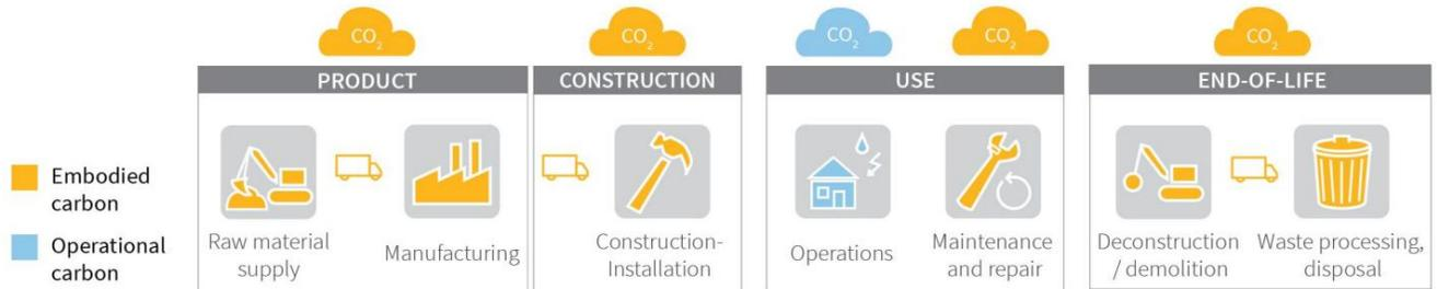
Figure 4. Embodied carbon (yellow) and operational carbon (blue) across the key life cycle stages of a building. *Image copyright to the Carbon Leadership Forum (CLF).*
